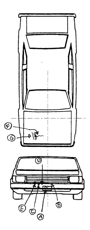
NOTES: Sketch all pedestrian contacts, include the size and depth in centimeters. Locate the pedestrian contacts from the intercept point of the centerline (lateral) and the front axles (longitudinal) in centimeters. Annotate observations which might be useful in reconstructing the accident (e.g., grass in tire bead, direction of striations, scuff on sidewalls, etc.).
